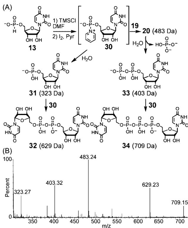
**Figure 2.** Mass spectral analysis of the reaction mixture obtained after conversion of *H*-phosphonate **13** to triphosphate **20**, using 3 equiv of TMSCl, followed by partial purification by gel filtration (Sephadex LH-20). Panel A: Structures of compounds detected by mass spectrometry. Panel B: Mass spectrum obtained with a Waters ZQ-4000 single quadrupole instrument using electrospray ionization (negative-ion mode).
